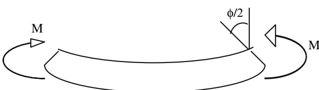
Fig. 15 End rotation due to bending of pipe
